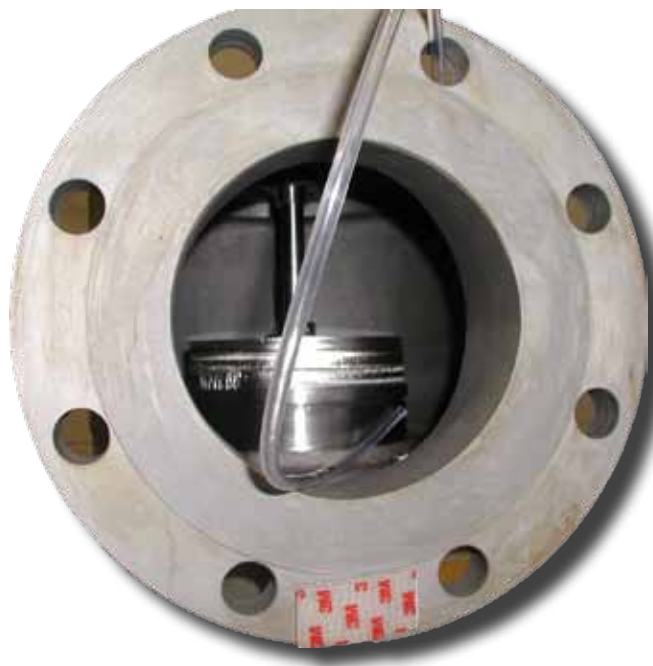
figure 1: Location of test probe in EPA Method 21 test setup located directly at sealing surface.
