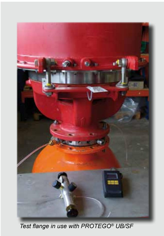
*Test flange in use with PROTEGO® UB/SF*
