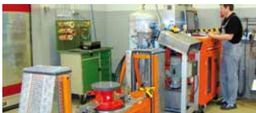
Figure 3: PROTEGO® vent valve testing
