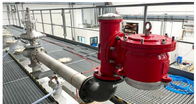
Test pilot-operated P/V-Relief Valve PROTEGO® VN-A-PCPF-S and a high-velocity Pressure Relief Valve PROTEGO® DE/S in combination with Vacuum Relief Valve PROTEGO® SV/E-S
