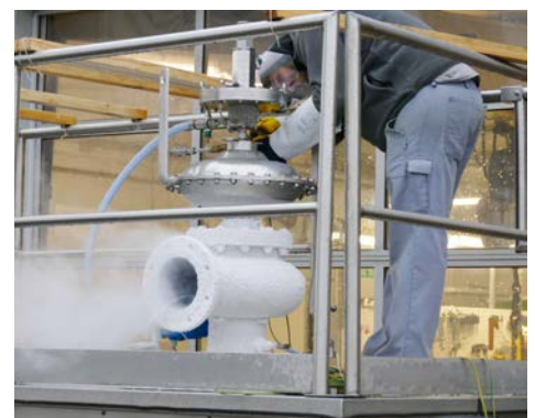
Functional test of PROTEGO® VN-A-PCPF at the Cryogenic test bench
