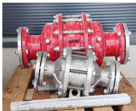
Tests of PROTEGO® DA-SB in the salt spray chamber
